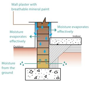
Wall with breathable mineral paint promotes free movement of moisture within the structure. Moisture evaporates, keeping wall dry and healthy.
