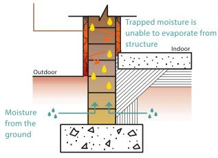
Wall with non-breathable paint traps moisture. The wall is constantly wet. Soaked plaster eventually spalls and paint blisters. PERMISSION REQUIRED
