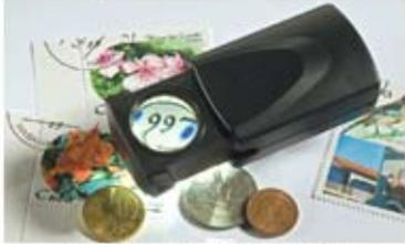
20x magnification. 1 LED light. Lens diameter: 21 mm. Operates with 3 x LR1130 batteries (included in delivery). Size: 54 x 34 x 23 mm.
