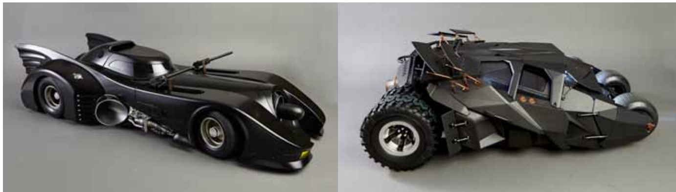
In 1989, BATMAN came back to the big screen after a hiatus of 23 years. The car he used was designed and produced by Tim Burton and Anton Furst. It was created from two Impala chassis and had a Chevy V8 engine. Collection of G&B Comics
